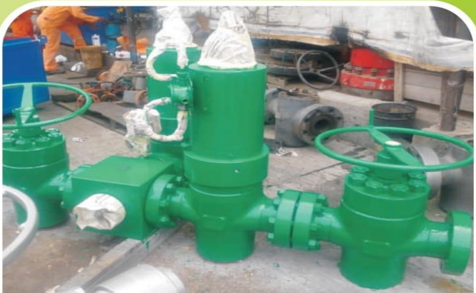
IBEWA 7 VALVE AFTER SERVICING
