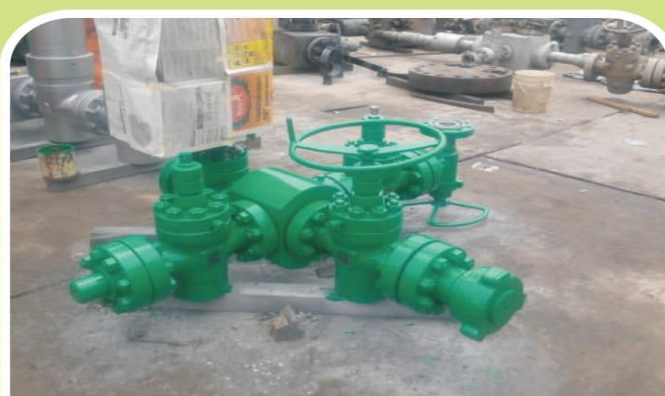
IBEWA 13 VALVE AFTER SERVICING
