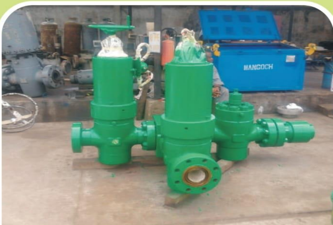
IBEWA 2B VALVE AFTER SERVICING
